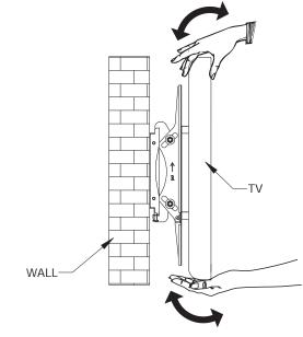
9-2. TV tilt bracket tension is preset at the factory. In case the tilt tension needs adjust, removethe TV from the mount; use a spanner wrench tightening or loosening the locknuts on the TV bracket.
